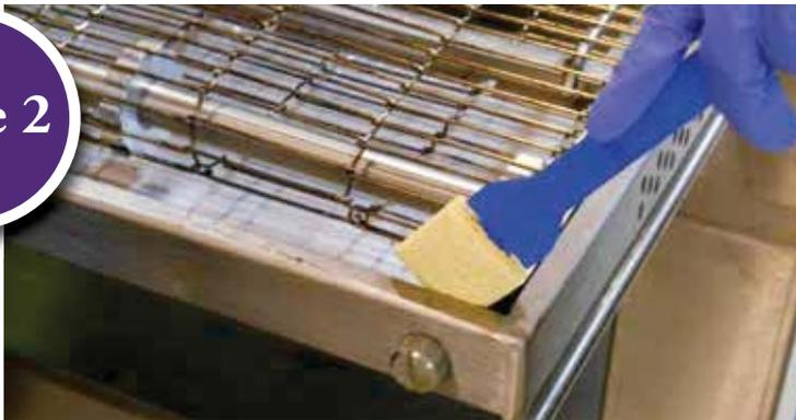
Nonfood contact areas in the plant that are closely adjacent to product contact surfaces. In general, this is the area where environmental contamination is most likely to affect the safety of the product (e.g., equipment framework, maintenance tools, drip shields, housings, etc.).
